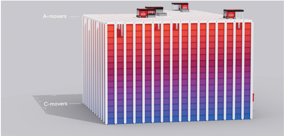
Figure 1. RCS/RS type AutoStore showing the principle of self sorting and ABC slotting (source: Autostore (2023)).
