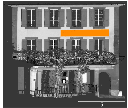
Fig. 5. Defined area (orange part) of a house facade. The point cloud is colored with the I_{\text{MCL},j,k}^s (Dataset 1, Z+F Imager 5016). (For interpretation of the references to color in this figure legend, the reader is referred to the web version of this article.)
