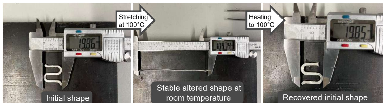
Figure 117: Demonstration of shape memory behavior of curved specimen of the polymer obtained by polymerizing LCM7 with the crosslinker CHTT and the chain extender HDT.
