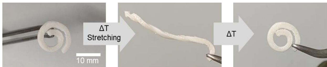
Figure 92: Shape memory test of a 3D printed specimen.
