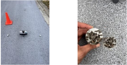
Figure 5. Traffic effect on adhesion of cool pavement.
