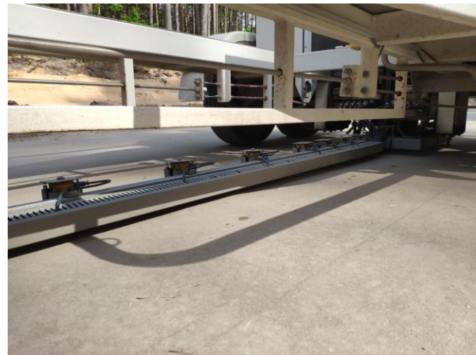
Figure 2. Pavement bearing capacity measurements with FWD.
