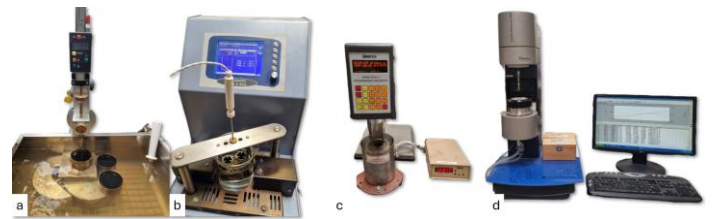
Figure 4. a) Penetration test b) Softening point test c) Viscometer Brookfield d) Dynamic Shear Rheometer (DSR)
