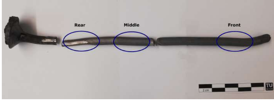
Figure 9: Rod of \text{Ti1ZrO}_2 , obtained from hot extrusion. Samples were taken from the marked sections (rear, middle, front).
