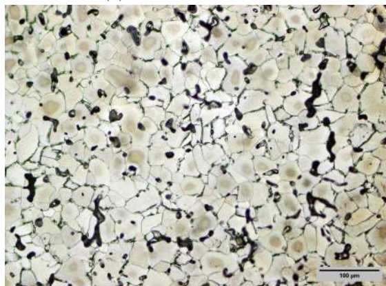
(e) \text{Ti}_{10}\text{ZrH}_2 as-sintered
