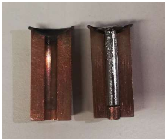
Figure 10: Sample for dilatometry measurements in cylindrical mold after melting in arc furnace
