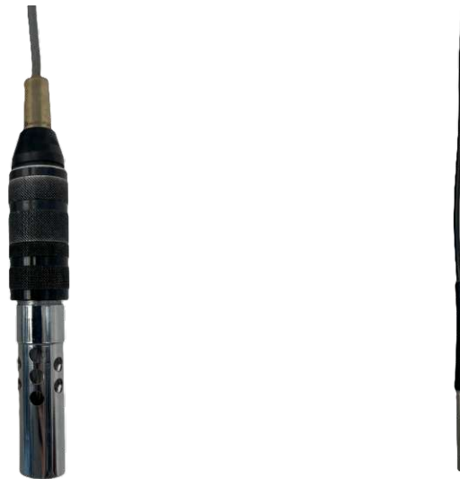
Figure 4.1.: Temperature sensors used at RTA. Left: Room temperature sensor. Right: Channel temperature sensors.
