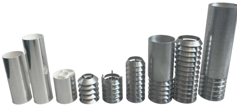
Figure 6.1.: Selection of tested radiation shield configurations for the XD33A sensor type.
