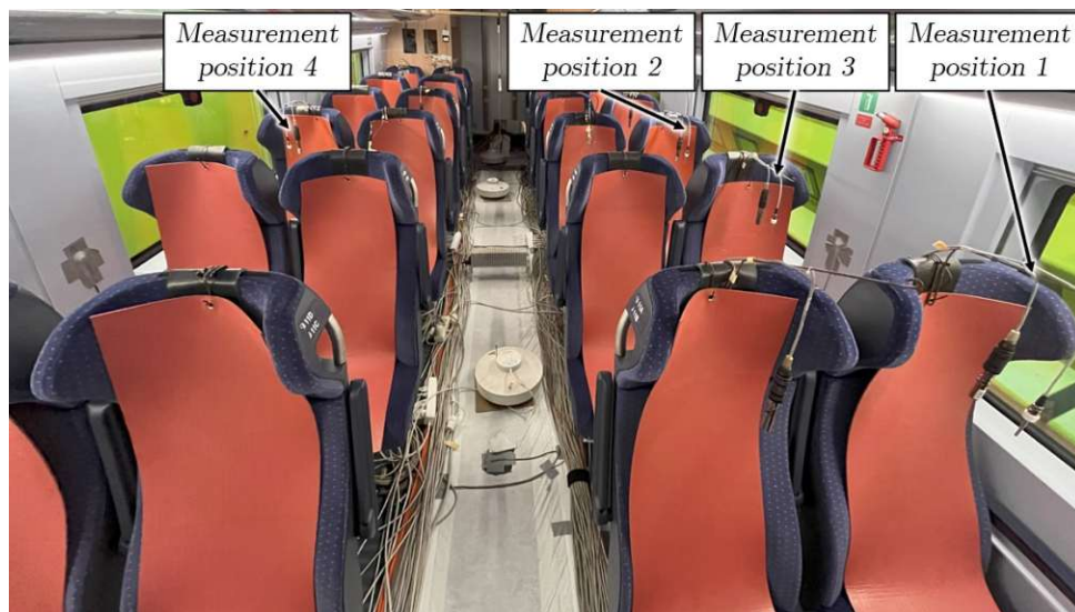
Figure 5.10.: Measurement positions in the rail vehicle. Measurement position 1 and 2 are identical. Measurement position 3 is not exposed to direct radiation. Measurement position 4 is on the shaded side of the vehicle. Photo taken in the Large Wind Tunnel (LWT).
