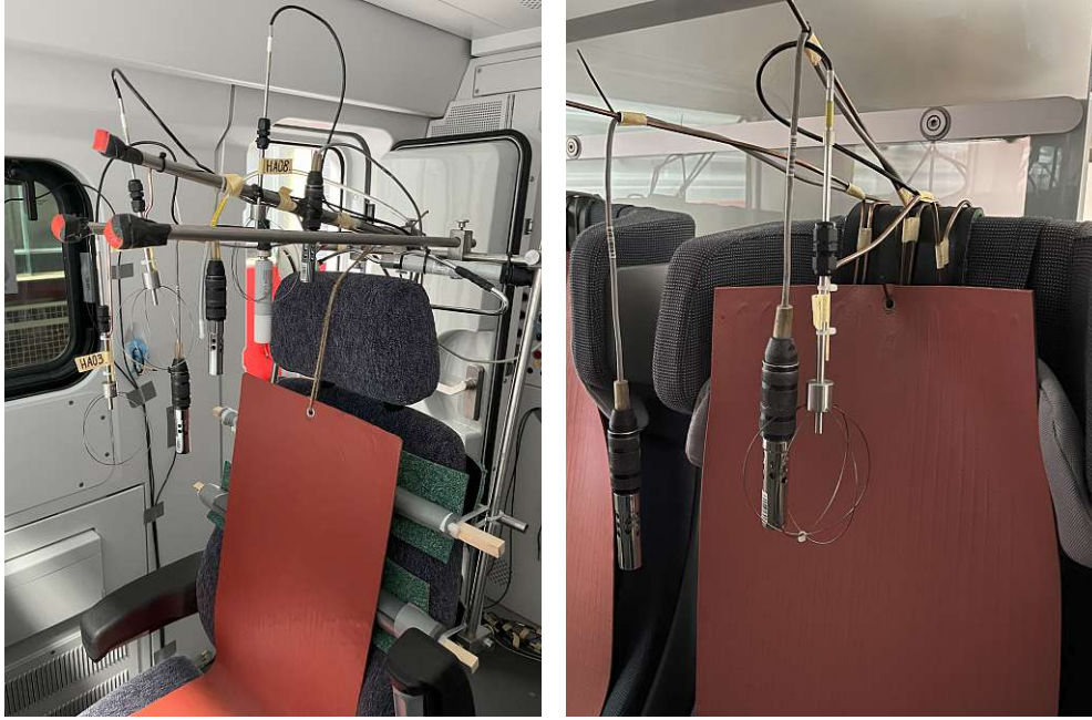
Figure 8.1.: Measurement setup in a long-distance railway vehicle. The anemometer probes are not fully extended to avoid potential damage. Left: Driver's cab. Right: Passenger compartment.
