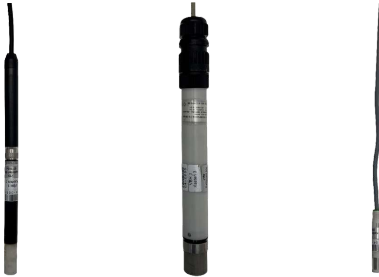
Figure 4.3.: Relative humidity sensors used at RTA. Left: XD33A. Middle: MP103A. Right: EE08.
