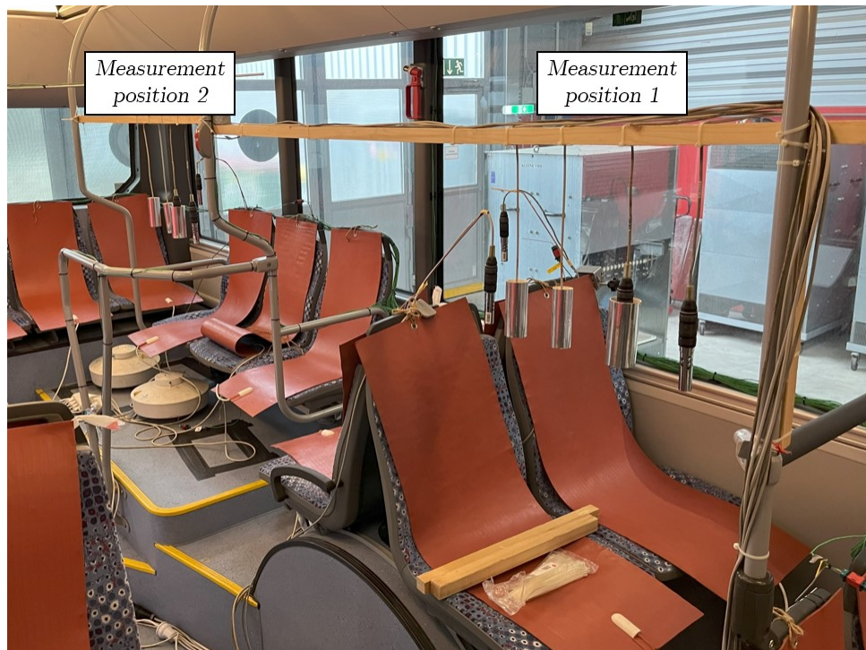
Figure 5.7.: Two identical measurement positions with measurement position 1 in the middle of the bus and measurement position 2 in the back of the bus. Photo taken in the preparation hall.
