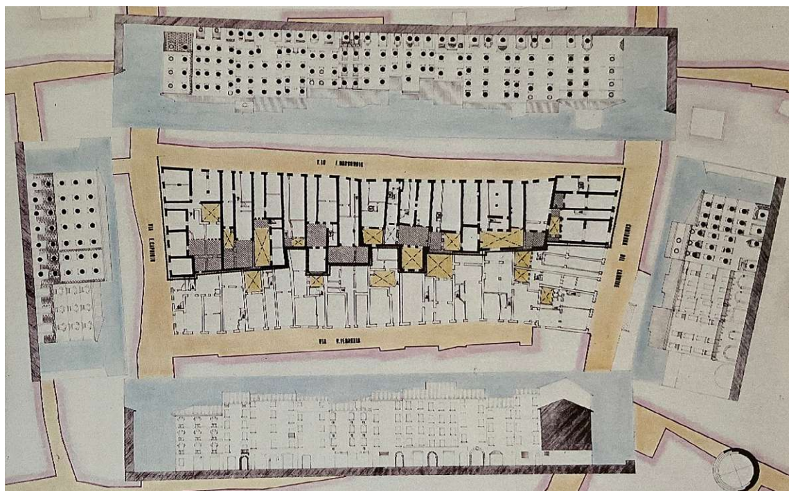
FIGURE 7 Recovery Plan for Vicolo Borgondio (Piano di Recupero di Vicolo Borgondio). Detail showing planimetric and façade restrictions. (Municipality of Brescia, Historic Centre Office, 1980. From Brescia moderna by Benevolo & Bettinelli, 1981, p. 417, CC BY-NC-ND)
