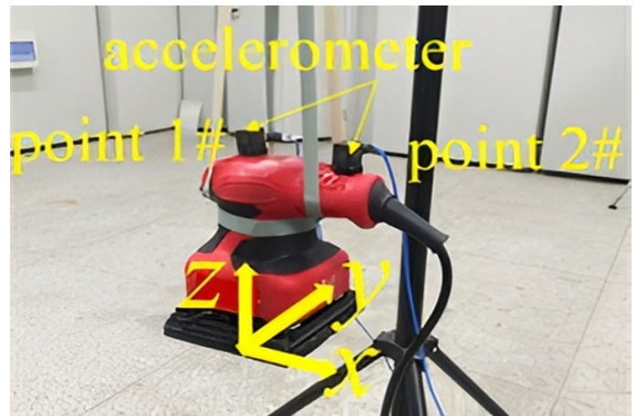
(b) Experiment to measure the acceleration of the housing[70].
