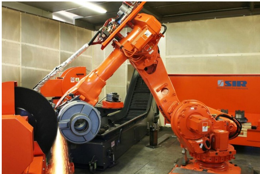
Figure 3.19: Machining changeable robotic workcell ( courtesy SIR SpA–Italy ) [20].
