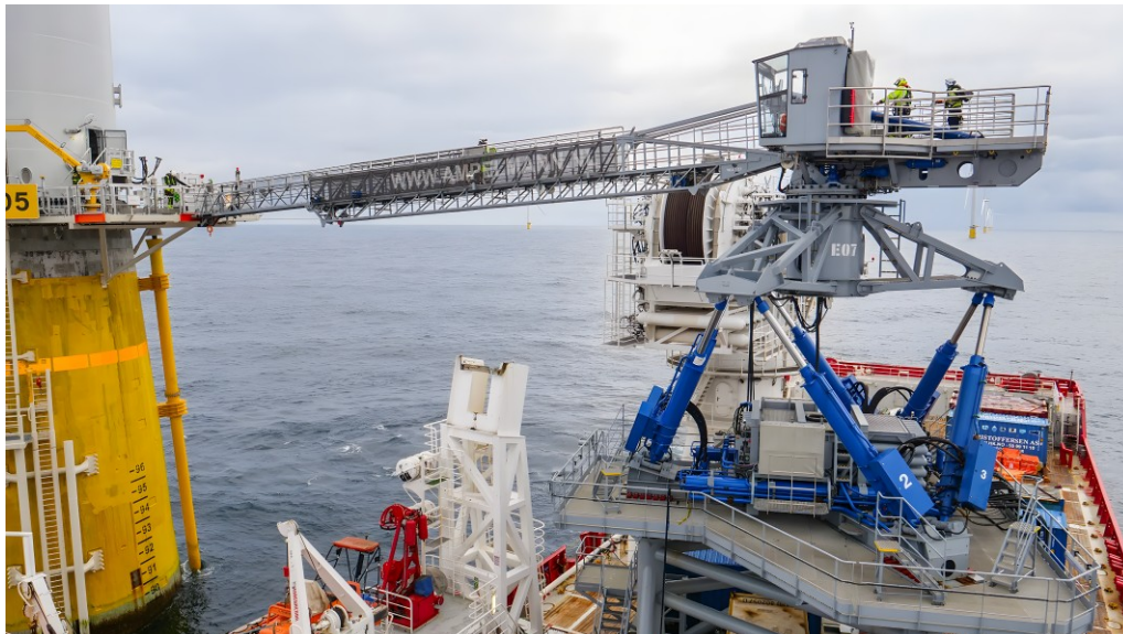
Figure 9.1: Ampelmann's hexapod system used for safe personnel transfer from an offshore construction site [103].
