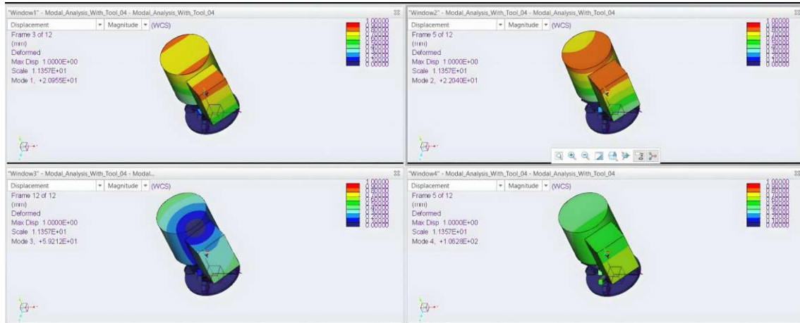
Figure 8.14: First four dominant frequencies along with their respective mode shapes for the Assembled Isolator.
