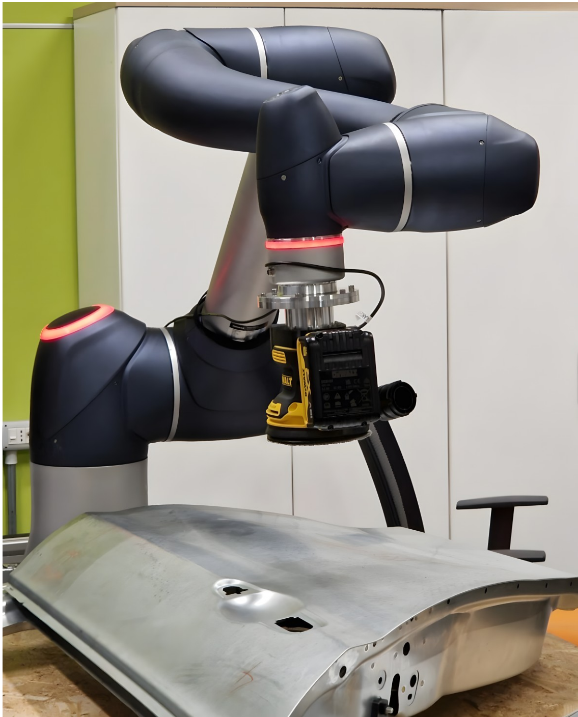
Figure 6.5: A Custom Autonomous Sanding Robot Workcell – End effector tool attached to the Doosan H2515 robot arm, along with the car front door.
