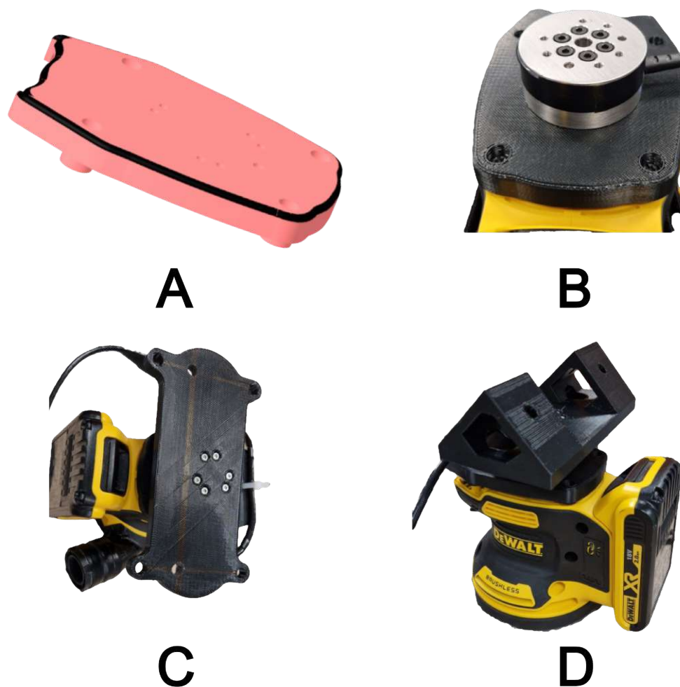
Figure 5.7: (a) CAD model of the modified Top cap for the tool, (b) Mounting of the FT sensor onto the modified 3D-printed cap, (c) A 3D-printed part for fixing the tool onto the aluminium extrusion, (d) A 3D-printed wedge-shaped part which is used to fix the tool in 45^\circ orientation.
