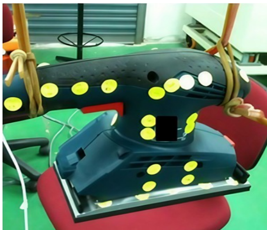
(a) The impact testing setup for the orbital sander in a free-free condition [69].
