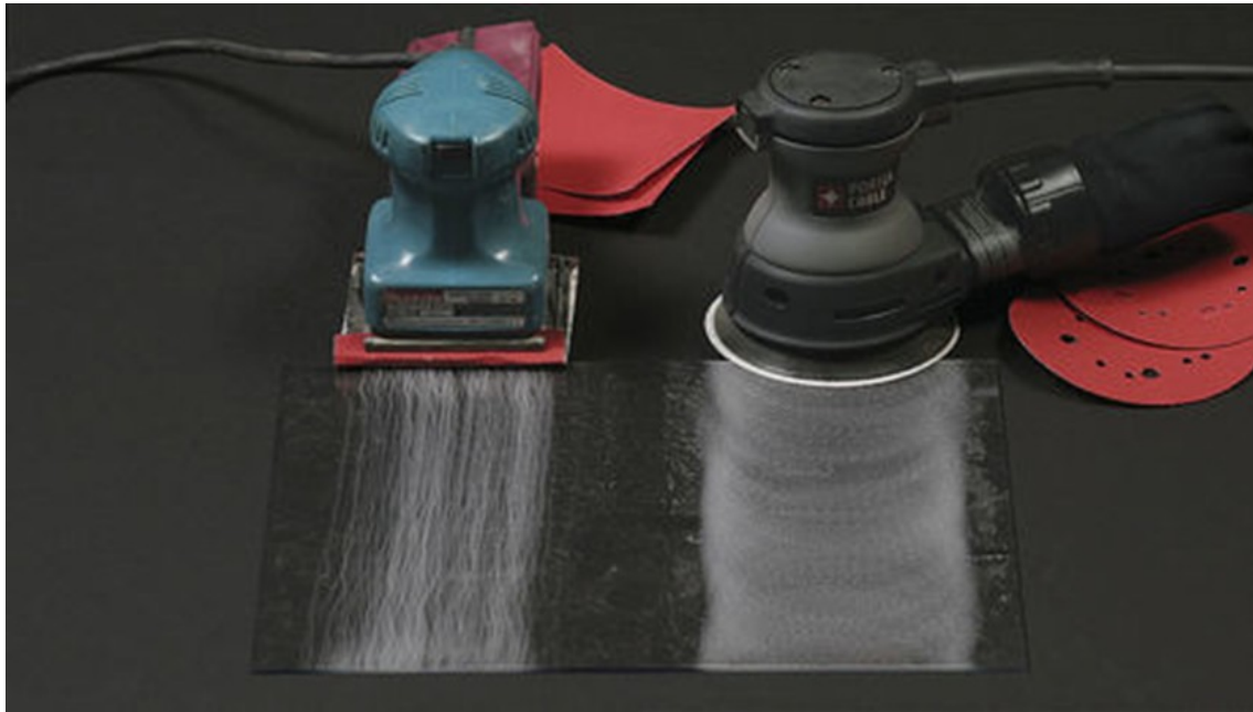
Figure 5.1: Comparison between orbital and random orbital sanding processes (Source: Fine Homebuilding [66]).
