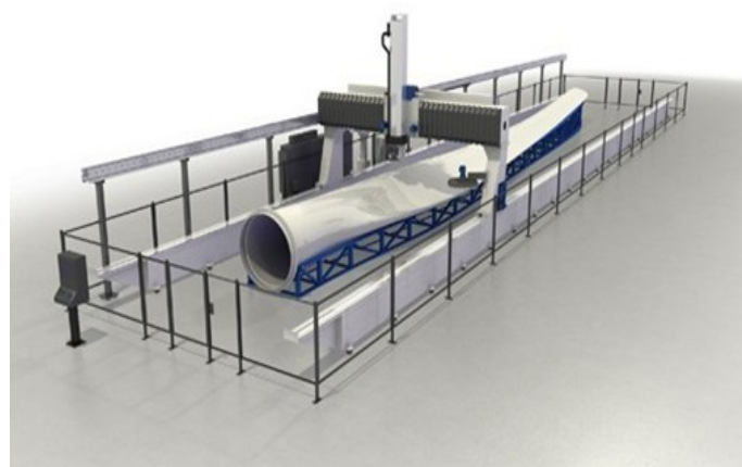
(b) Large 5-axis Agile Gantry System that is used in Wind blade manufacturing [19].
