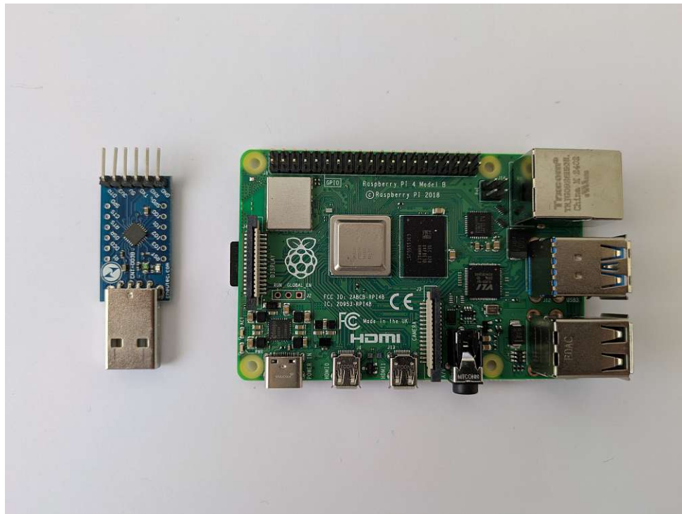
Figure 3.1: Image of Raspberry Pi 4 Model B with USB to TTL converter
