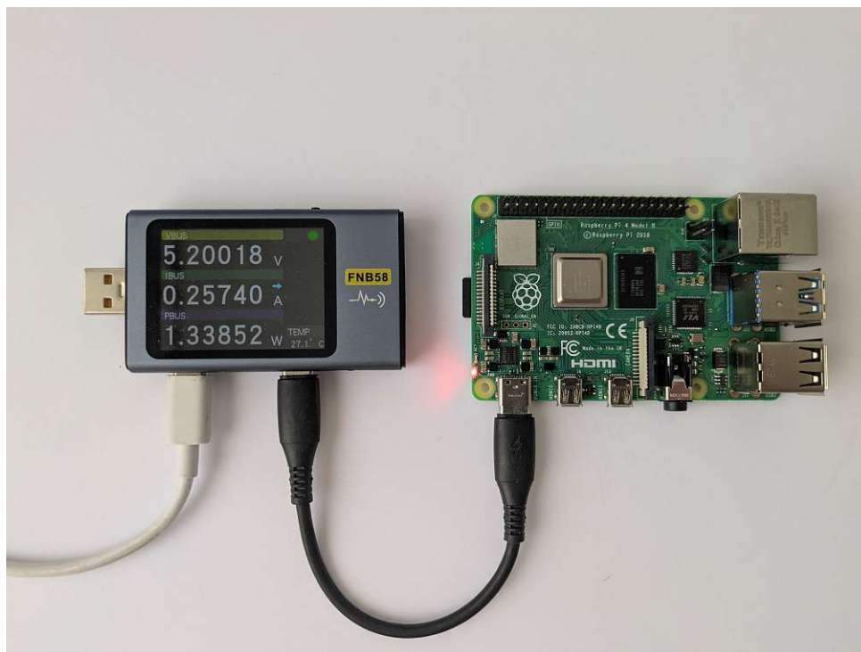
Figure 3.2: Image of the test setup with FNB58 and Raspberry Pi 4 Model B
