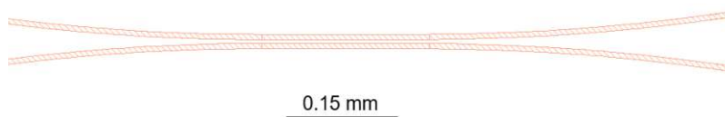
Figure 8.5: Close up of the directional coupling structure for 50/50 coupling of 493 nm laser light. The coupling length was calculated to be 8.1 \mu\text{m} .
