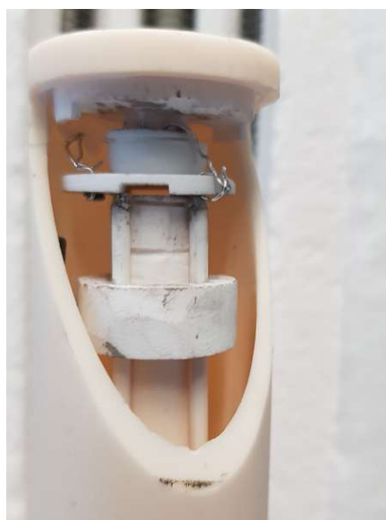
Figure 8: Mounted titration cell on a self-made sample stage.
