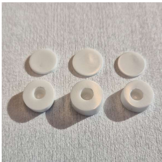
Figure 6: Sintered YSZ pellets: Above the thin lids and below the cells with the milled cavity.
