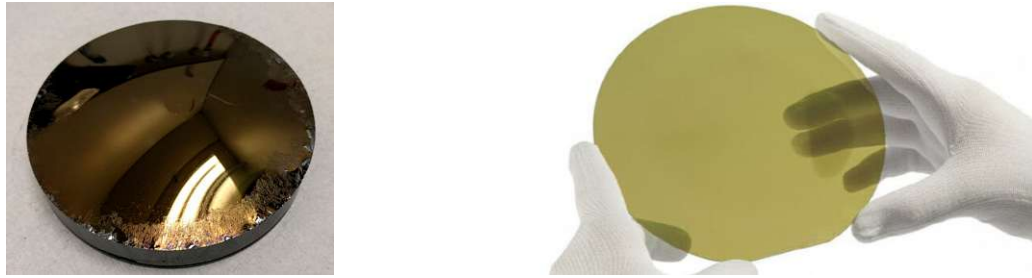
Figure 2.1.3: Left: silicon carbide boule grown using physical vapor transport [50]. Right: 4H-SiC wafer with a CVD-grown epitaxial layer ready for processing [51]. Note the transparency to optical light.
