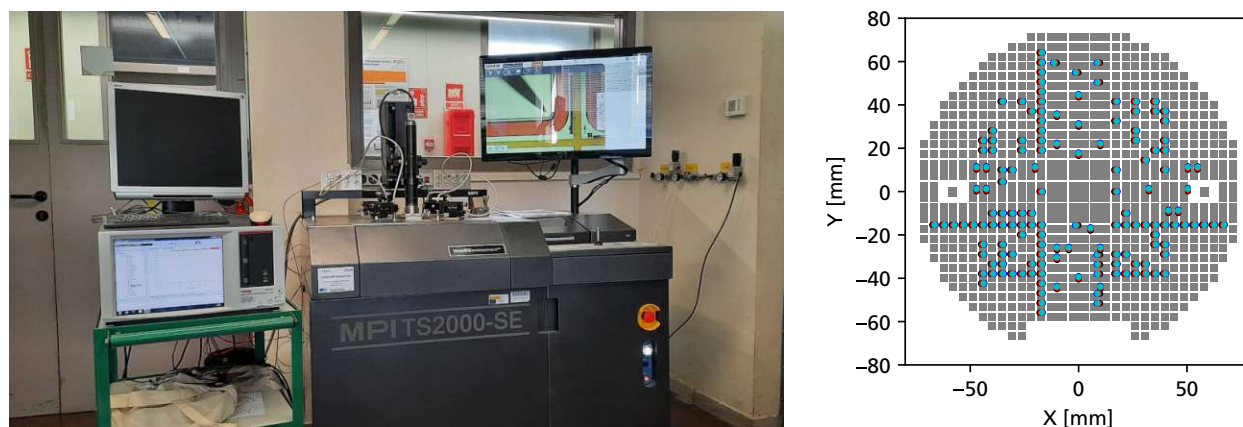
Figure 6.3.2: Left: Semi-automatic probe station MPI TS2000-SE measuring 4H-SiC PiN diodes in the characterization lab at IMB-CNM, Barcelona. Left of the probe station, a Keithley K4200 semiconductor analyzer is visible, conducting C-V measurements. Because 4H-SiC is insensitive to visible light, measurements can be conducted simultaneously with visual inspection. Right: On-wafer coordinates of process quality control structures extracted from the mask layout. Each colored dot corresponds either to a Van-der-Pauw or a cross-Kelvin bridge structure. The gray rectangles indicate the individual dies of the wafer.
