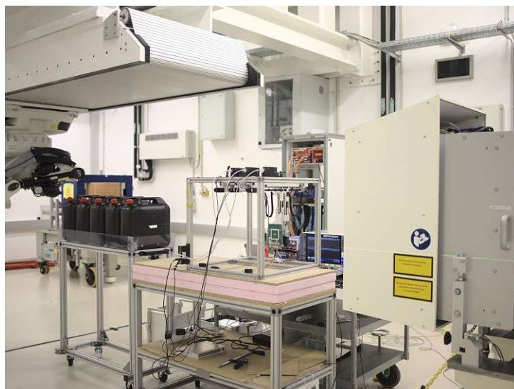
Figure 4.4.1: IR1 Beamline at MedAustron. The beam enters from the right side through the nozzle containing the dose-delivery system. In the isocenter, a detector mounted on a UCSC LGAD board is visible. Photo credit: Simon Waid.
