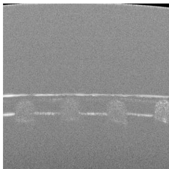
Figure 3.3: Deflection image of the coated membrane during dynamic loading (Trial 4)
