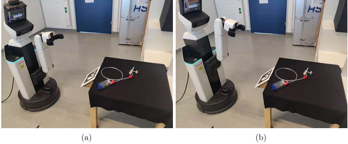
Figure 4.3: First two gripper poses during the experiment, where an image is captured at each pose. (a) Initial pose at the start of the experiment. (b) Predefined pose reached to capture the scene from an alternative viewpoint.
