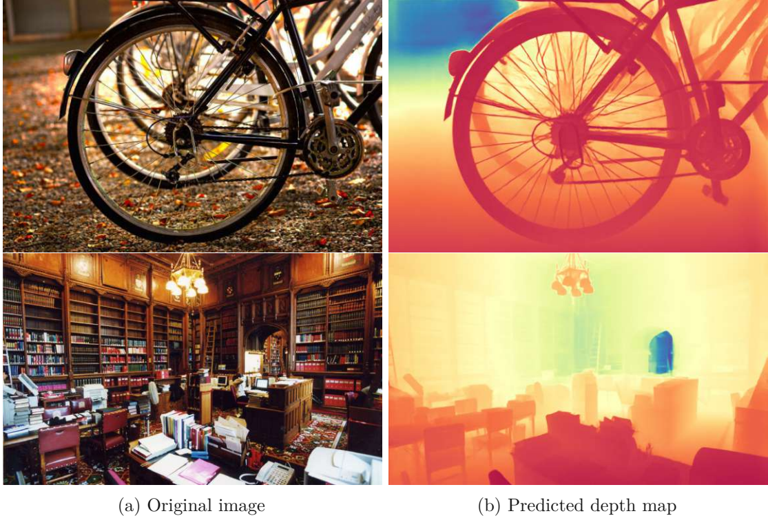
Figure 3.2: Qualitative results of Depth Anything V2 [4]. (a) Input RGB images. (b) Corresponding monocular depth predictions, where red denotes closer regions and blue denotes farther regions relative to the camera. The examples illustrate the model’s ability to recover fine-grained depth structure from a single image.
