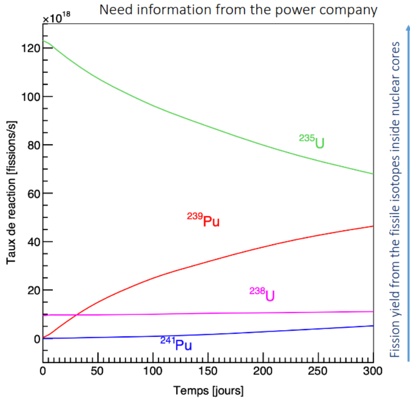
Figure 1.7. Time evolution of isotope content in the fuel mixture over a cycle of 300 days starting with fresh fuel (No Plutonium from previous cycles). Figure from [54].
