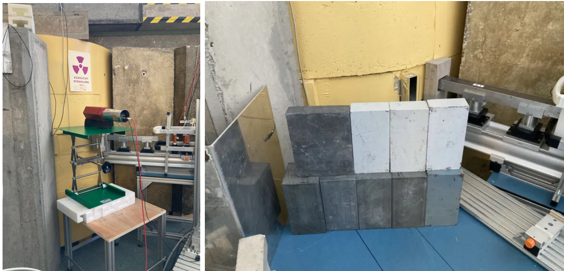
Figure 8.3. Left: Scan of the background rate along the height of the monochromator shielding. Right: Test using lead bricks placed near the monochromator shielding to shield the CRAB area from emitted radiations.
