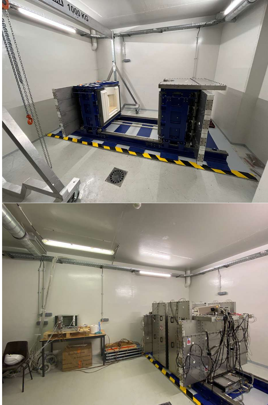
Figure 3.25. Pictures of the Muon Veto installation and cabling at the VNS.
