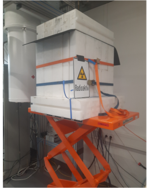
Figure 6.1. Left: Scheme of the experimental setup including the cryostat, the cryogenic detector and the portable neutron source. Figure from [121]. Right: Picture of the experimental setup with the ^{252}\text{Cf} portable thermal neutron source.
