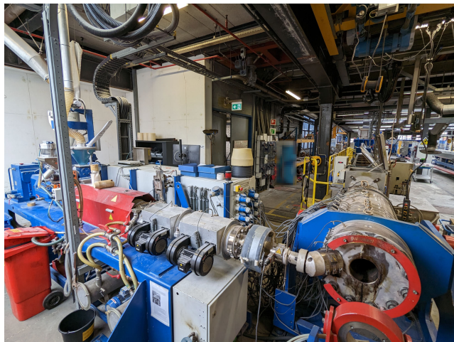
FIGURE 2. Setup of the bi-oriented PVC production line with gravimetric dosing system, extruder, adapter, die head, cooling zones and subsequent drawing section (left to right).
