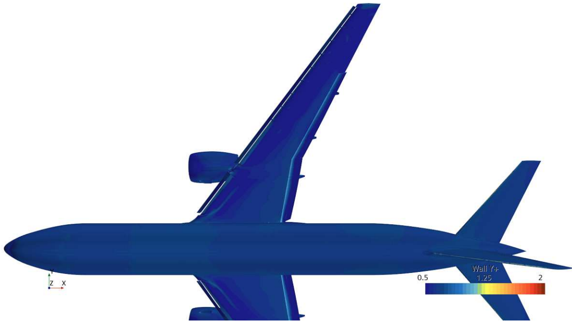
Figure 3.14: Wall y^+ values for the first cell
