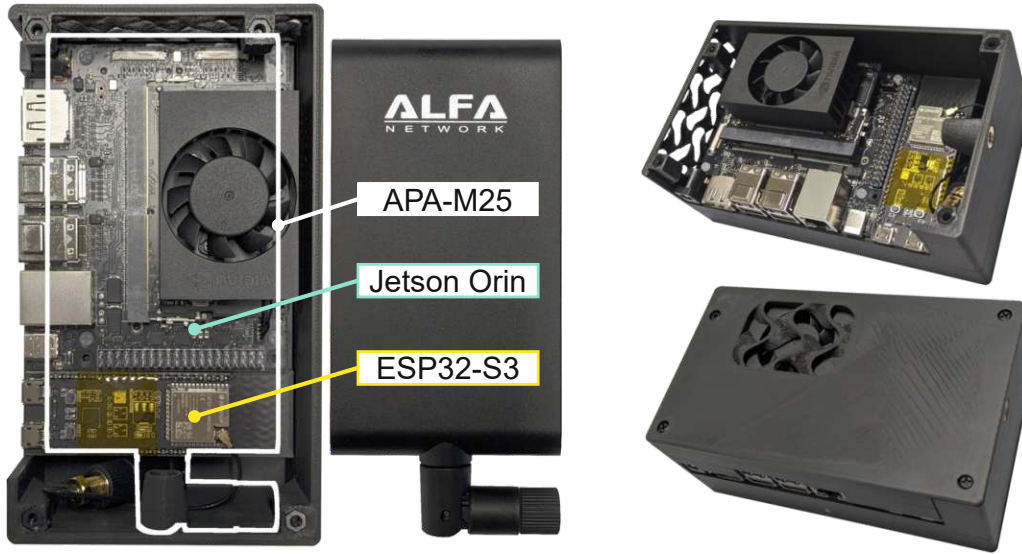
Figure 4.6: Overview of system \mathcal{D} , showing internal components comprising ESP32-S3-DevKitC-1 module, ALFA Network APA-M25 directional panel antenna, and Nvidia Jetson Orin Nano developer kit. [49]
