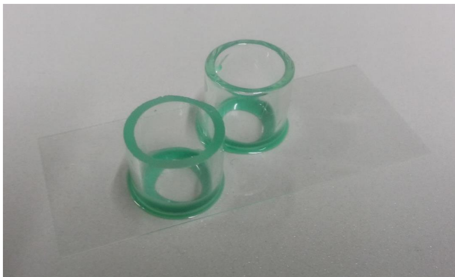
Figure 83. Set up for the surface modifications on glass cover slips
