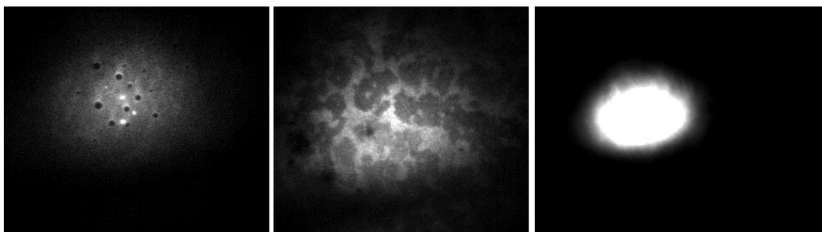
Figure 95. Comparison of the TIRFM images of the functionalization with APTES in 3 wt% (left), 4 wt% (middle) and 5 wt% solution (right)
