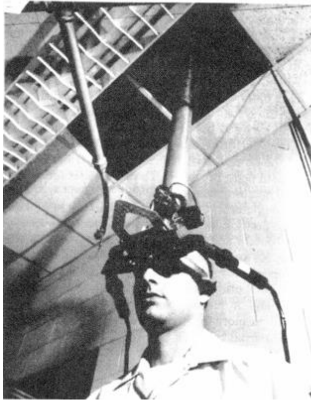
Figure 4: The “Sword of Damocles”, the first head-mounted display for virtual reality, developed by Ivan Sutherland (Sutherland, 1968)
