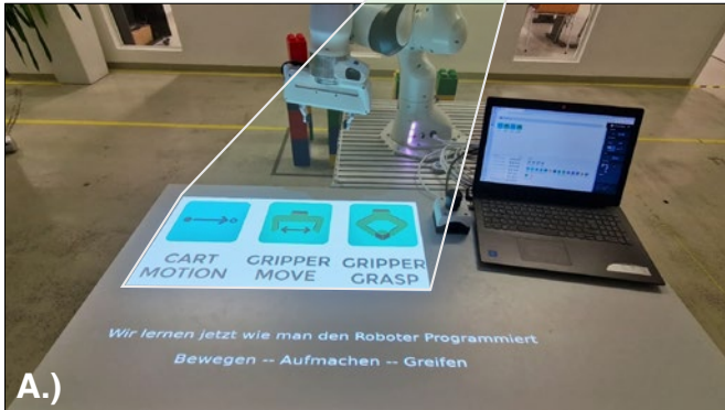
Figure 2: Visual depiction of selected use cases: A.) learning how to program a collaborative robot with SAR instructions, deployed in lab settings; B.) instructional videos integrated in the workspace via the example of operating an industrial buzz mill; C.) interactive projections, depicted via the example of choosing the right buzz saw tool according to material properties.
