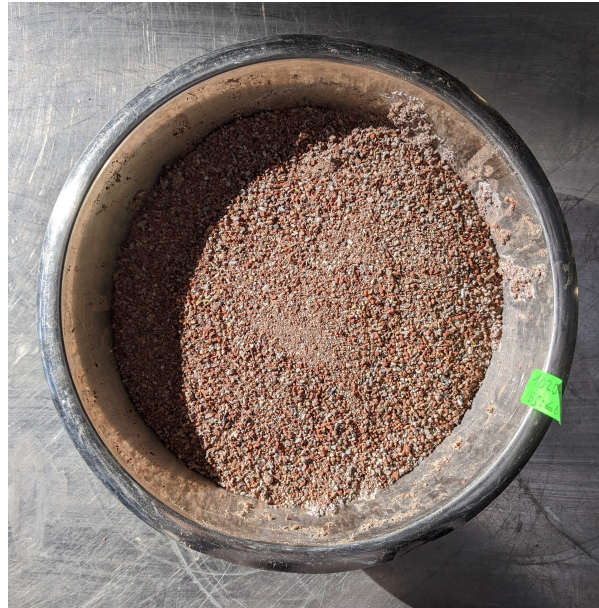
Figure 3. The crushed and washed demolition waste after drying.
