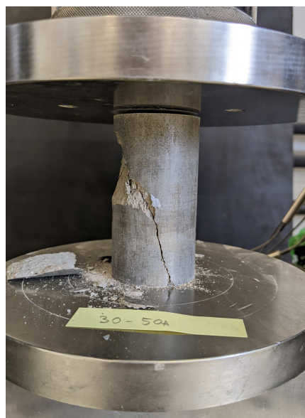
Figure 12. Failure pattern after compressive strength test in approximately two-thirds of the cases.
