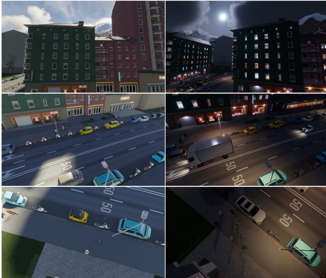
Figure 5.2: In-game movement example of a single PTZ camera at a fixed location. The camera is rotated in a controlled way during the day and at night.
