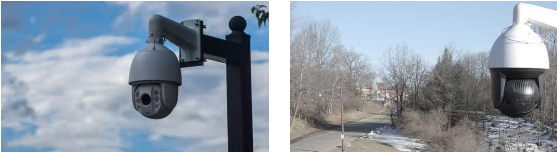
Figure 1.2: Left: front view of a PTZ camera mounted on a pole. Right: back view, also showing parts of the camera’s FoV. Images from [Gmb25, Tea23].
