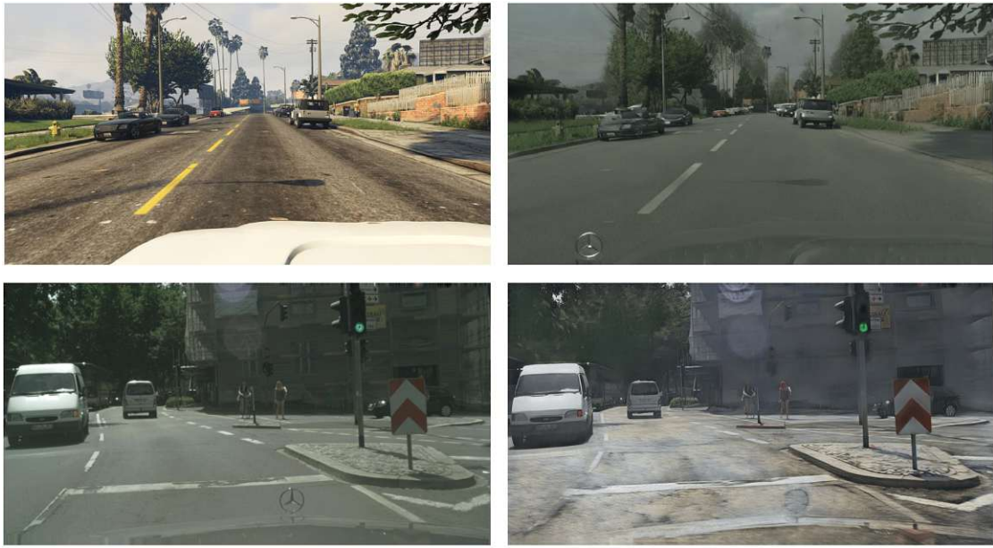
Figure 3.5: Example of GAN-based domain adaptation via CyCADA. The model transforms an image from GTA V, a computer game, to the real-world Cityscapes [COR + 16] dataset (top), and performs the reverse transformation from Cityscapes to GTA V style (bottom). Images source: [HTP + 18] page 6
