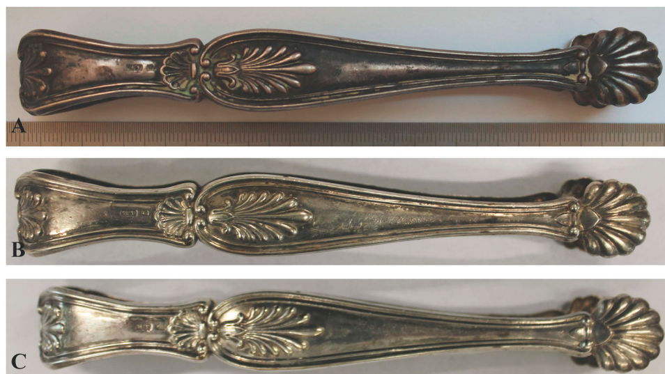
Figure 5. Naturally aged silver tongs. (a) untreated; (b) treated with the electrolytic pencil (electrolyte with pH4.5) equipped with the clean room sponge tip, at -2.5 V for 20 min, and consecutively at -3.0 V for 5 min; (c) Additional treatment with the electrolytic pencil equipped with a felt tip at -4.0 V for 10 min.
