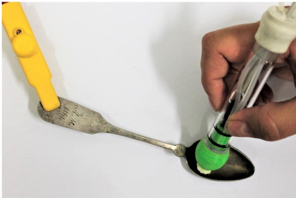
Figure 3. Electrolytic pencil application at a silver spoon. The object is contacted as the working electrode.
