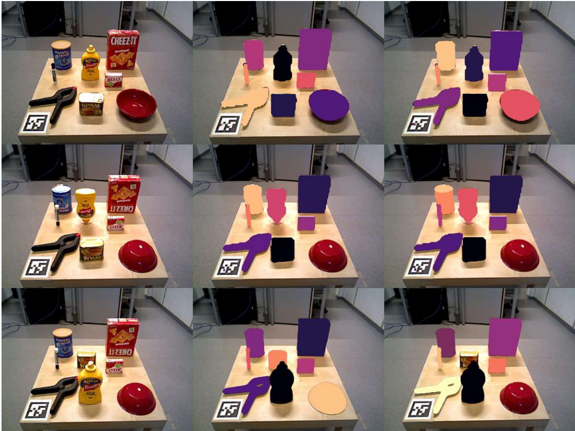
Figure 4.9: Representative test scenes, with the second column illustrating CNOS segmentations and the third column presenting SAM-6D ISM segmentations. The segmentations in the first and second rows are generated using FastSAM, whereas those in the final row are produced using SAM.
