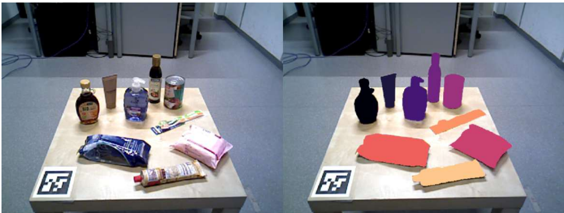
Figure 4.10: Representative segmentation outcome obtained using the most robust CNOS/SAM configuration on MANiBOT objects.
