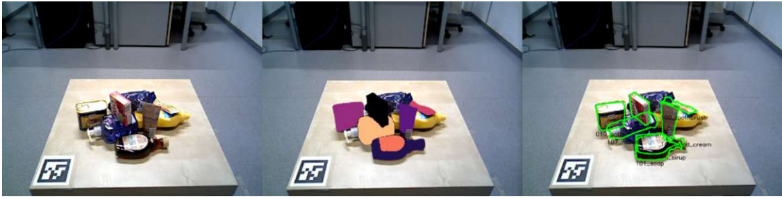
Figure 4.15: Illustrative example of one of the six exploratory multi-object scenes with overlapping object boundaries, including object segmentations and their corresponding 6-DoF poses projected onto the image plane. The visualization highlights recurrent failure modes: mutual misclassification between "soap" and "razors", duplicate segmentation of a single object with two distinct class labels, as exemplified by "ahorn_sirup", and missing segmentations for objects with more strongly overlapping boundaries.
