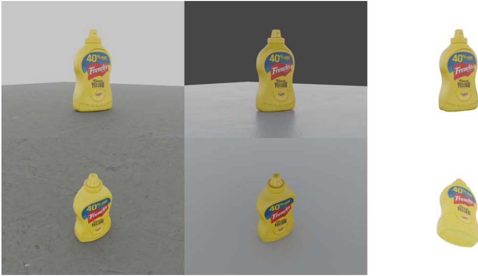
Figure 4.1: YCB-V object rendering with high/low feature surface and extracted segmented RGB masks; rendering angles of 0^\circ , 45^\circ , and -45^\circ to the horizontal plane.
