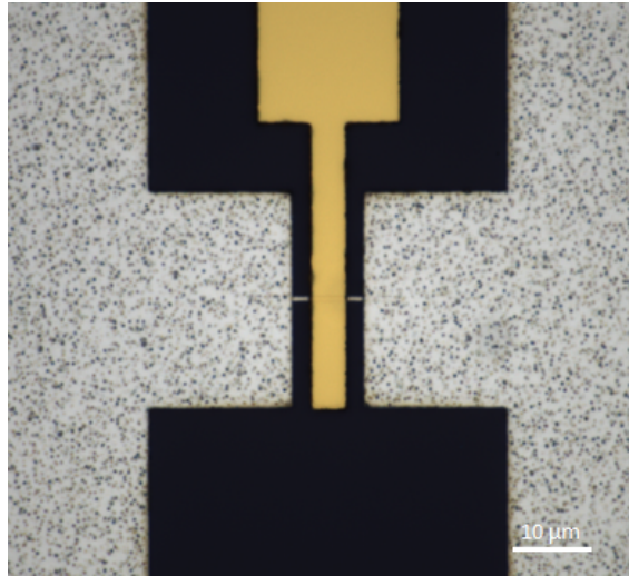
Figure 4.2: STG device with Au top-gate captured by optical microscope.
