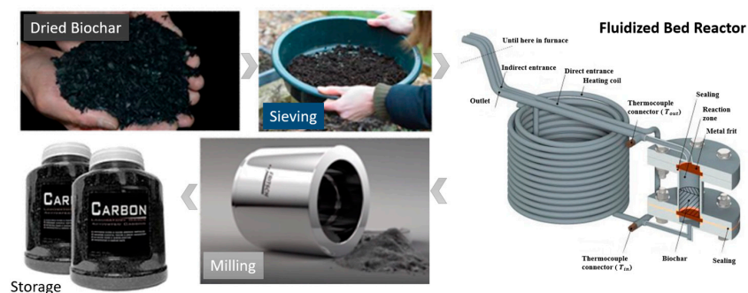
Figure 5. Steps of the biochar preparation process and the laboratory-scale fluidized bed reactor used for activation [18].
