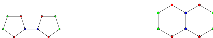
Figure 2.3: The molecules bicyclopentyl (left) and decalin (right) which cannot be distinguished by WL algorithm and thus by any MPNN. Node colours are the result of the WL node colouring algorithm. Figure adapted from Sato [2020].
