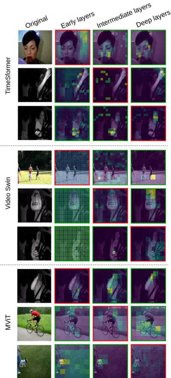
Figure 5.2: Visualization of the attention maps produced by the highest and lowest relevance heads for TimeSformer, Video Swin and MViT. Red boxes indicate the lowest relevance heads within the corresponding layers, while green boxes indicate the highest relevance heads within the corresponding layers. Early layers refer to the first layer for TimeSformer, and first two layers for both Video Swin and MViT, while deep layers correspond to the last one in TimeSformer, and last two layers in Video Swin and MViT. Intermediate layers encompass those in between. Colormap: viridis (dark blue: low attention, bright yellow: high attention). Best viewed in color.
