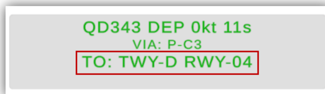
Figure 3.12: Plane information of a departing plane, showing assigned runway (RWY-04) and intersection (TWY-D) to depart.
