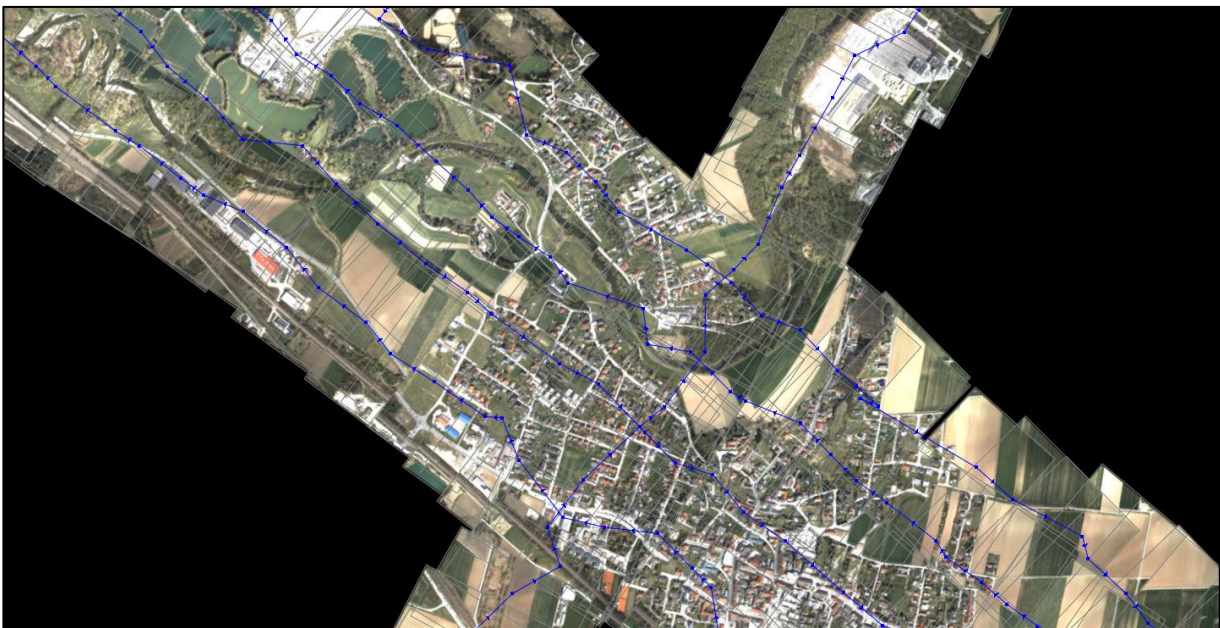
Figure 10: Strip deformations resulting from a failed Aerotriangulation.
