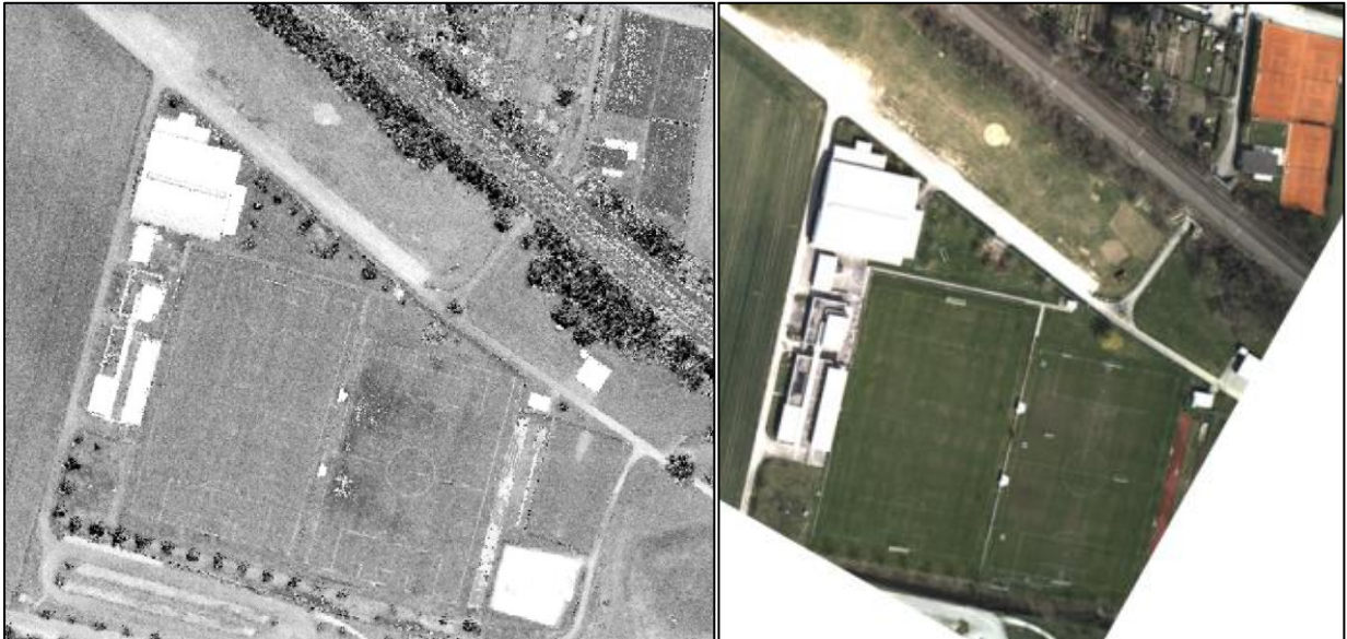
Figure 7: Comparison of an aerial RGB image (right) and an Amplitude map derived from ALB data. Though the aerial image shows a clearly better resolution, most major objects can be identified in both representations – even the lines on the soccer field can be recognized.
