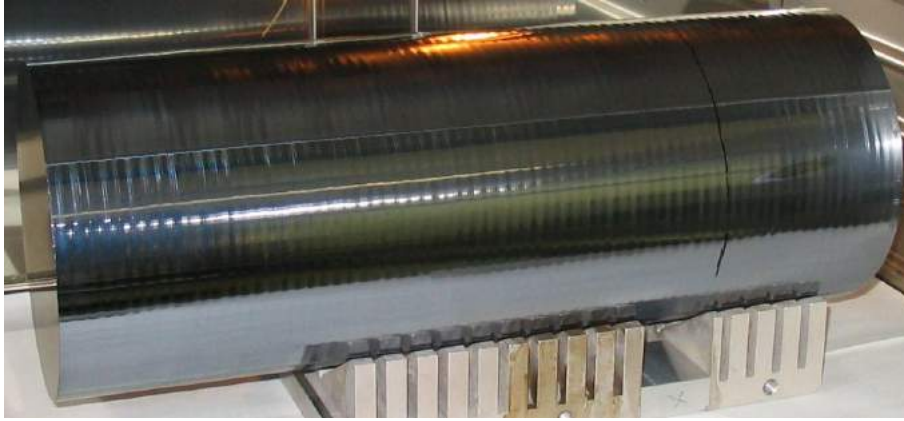
Figure 3.2.: Silicon perfect crystal ingot before cutting at PTB.
