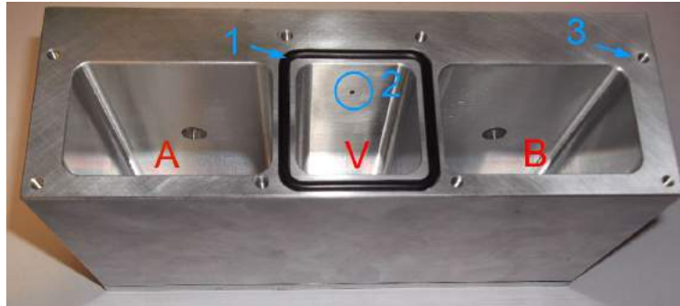
Figure 4.6.: Al chamber system without outer walls. (A)(B) Air chambers ( 65 \times 94 \times 40 \text{ mm}^3 ), (V) vacuum chamber ( 40 \times 94 \times 40 \text{ mm}^3 , wall thickness to (A)/(B) is 8 mm). (1) Vacuum sealing ring, (2) connection to the vacuum system and He-inlet ( \text{Ø}5 \text{ mm} hole), (3) screw hole for mounting Al walls.
