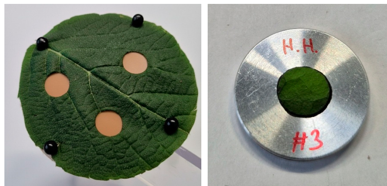
Figure 4. Pinned leaf with punched-out holes for sampling (left) and samples glued with conductive carbon adhesive for SEM analysis (right); technical replicates n = 6 .
