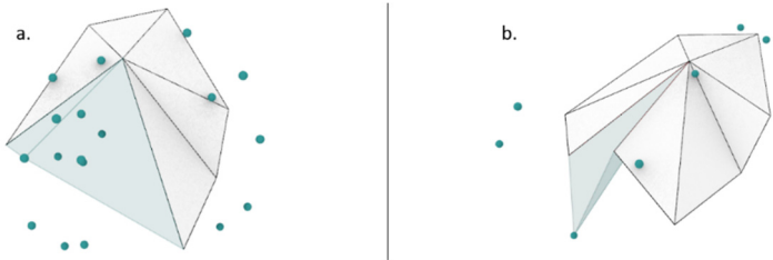
Figure 6: Closing fan-shaped assemblies with two adjacent panels will lead to coherent (a) or eccentric (b) results according to the size of the solution space.
