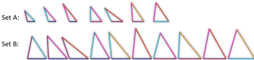
Figure 4: The number of triangles that can be generated varies with the chosen set of edge lengths (Set A: 20, 30, 40, 50, 60cm; Set B: 50, 60, 70, 80, 90cm edge length)
