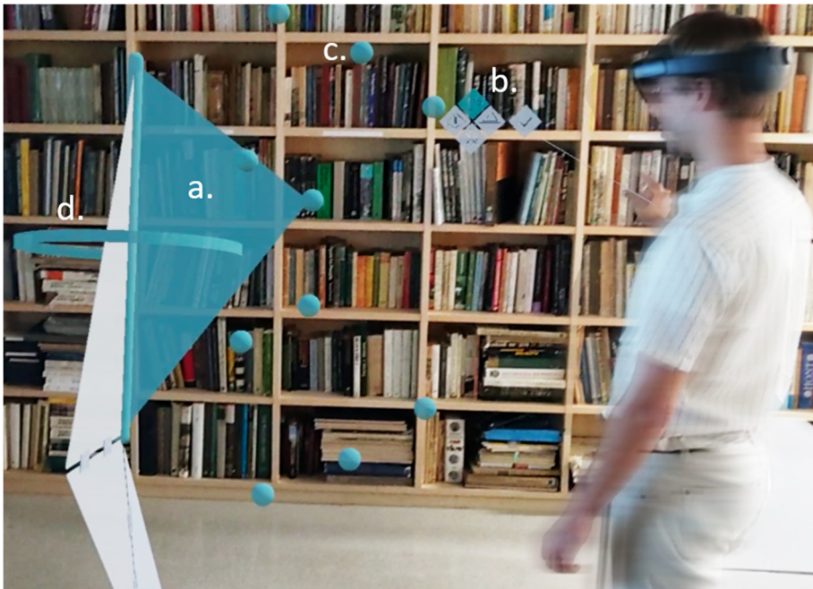
Figure 3: Users can interact with the structure through the AR interface (a), and use a control panel to choose between four actions (b), and explore the design space (c and d).
