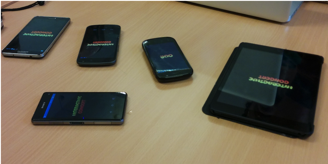
Figure 5.2: Smartphones reacting on a high frequency sound ID via a sequence of pictures.
