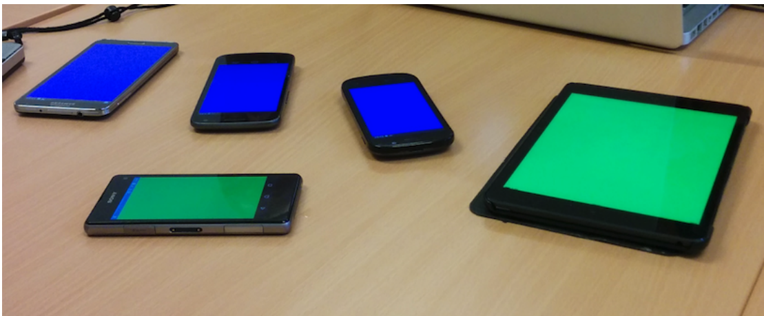
Figure 5.3: Smartphones reacting on a high frequency sound ID changing the display colour.
