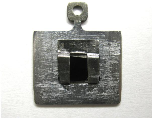
Figure 6.2: Sample crystal of  $\text{SrTiO}_3$  as used in the XPS/XANES experiments, mounted on a conducting sample holder.
