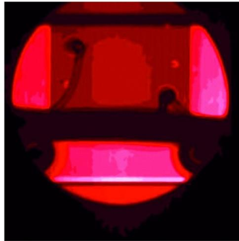
**Figure 5.6.2** *Left:* Processed image from scintillator detector dried at 70°C with  $\text{N}_2$  to purge water from the channels. **Right:** Processed image of the cell with 30% humidity. The MEA is located in the square region in the middle of the image. High intensities indicate thicker water regions (red color). The color mapping helps to show changes in water content, not easily resolved in gray scale images of the human eye just as in the figure 5.6.1.
