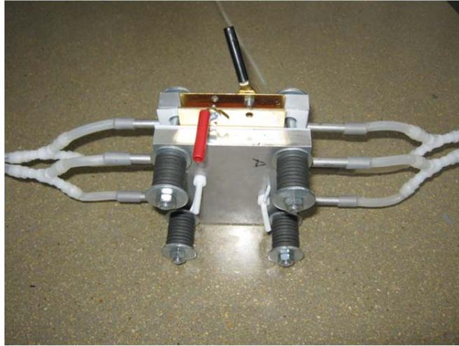
**Figure 5.5.3** *View of the stationary fuel cell used in radiography measurements at NR II station.*
