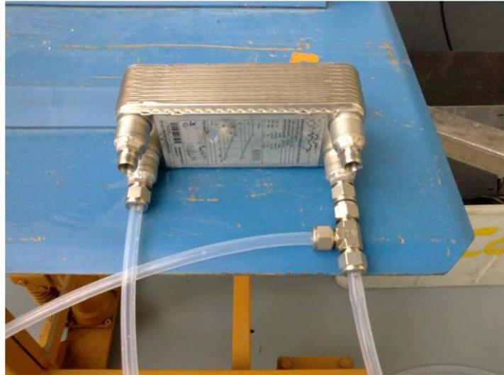
**Figure 6.4.1** *The heat plate exchanger used in the experiment at NR II station at ATI produced from Alpha Laval Company.*
