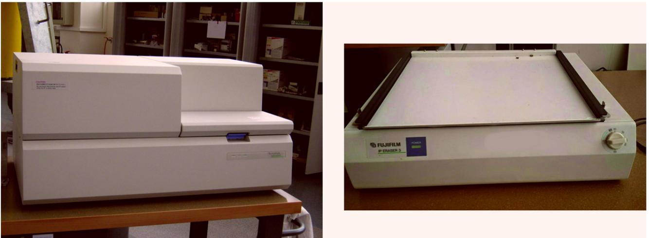
**Figure 2.4.2** The BAS-5000 scanner and the eraser device at NR-II station at Atominstytut.
