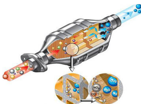
Figure 1.1: Schematic illustration of Three Way Catalytic Converter. Adapted from ref. [18].
