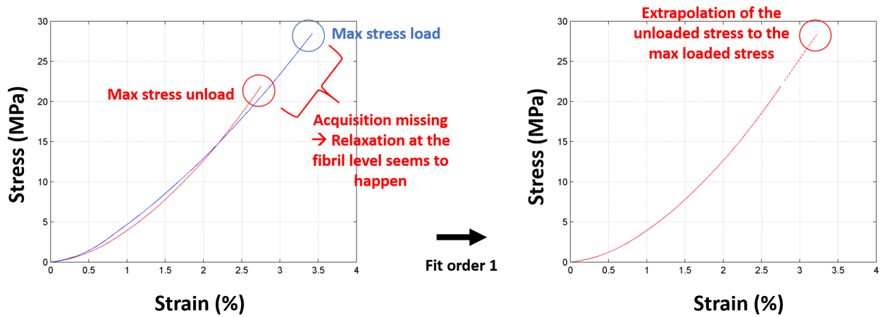
Figure 5.19: Estimation of the non acquired unloading data points with a polynomial fit order 1 for the unloading curve in 2.6M PEG
