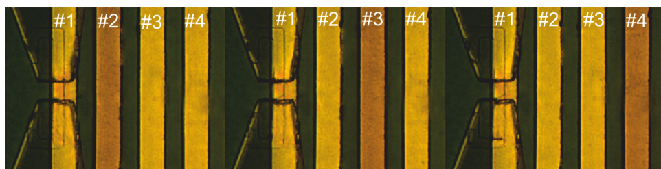
Figure 7.2: Sequential actuations of the MCs and manipulation of the MNs as a pre-concentration step. MNs are attracted to the current carrying MCs and are finally concentrated on MC #2.
