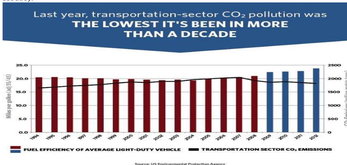
**Figure 6:** US transport & LDV - Trends of fuel efficiency [miles/gallon] and CO<sub>2</sub> emissions [mil.t]. [7]
