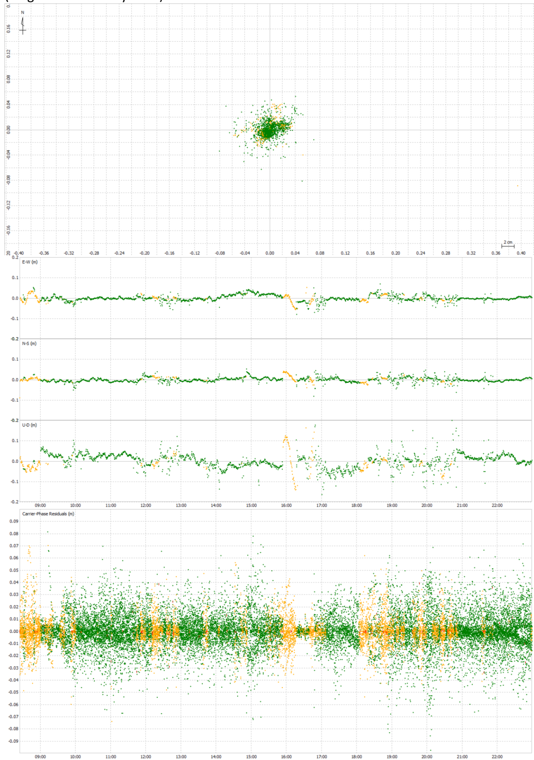
7.2 km baseline, L1/L2 LC, time series of position results and carrier phase residuals (fix-green and float-yellow).
