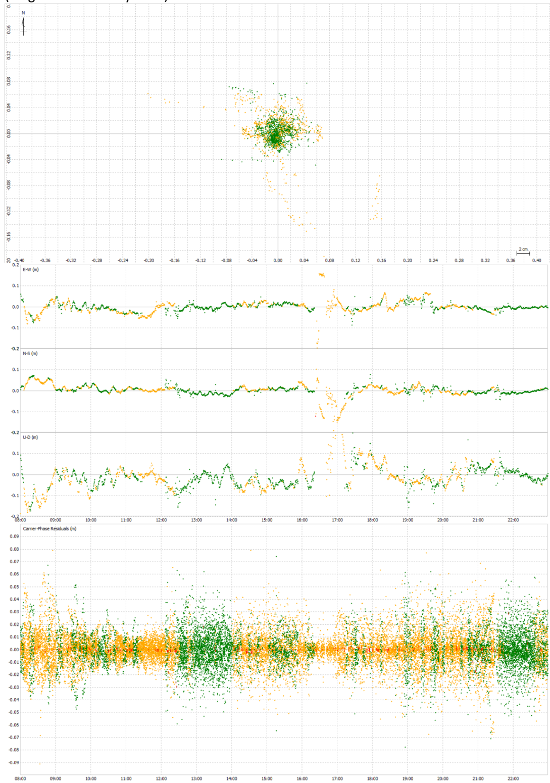
25.9 km baseline, L1/L2 LC, time series of position results and carrier phase residuals (fix-green and float-yellow).
