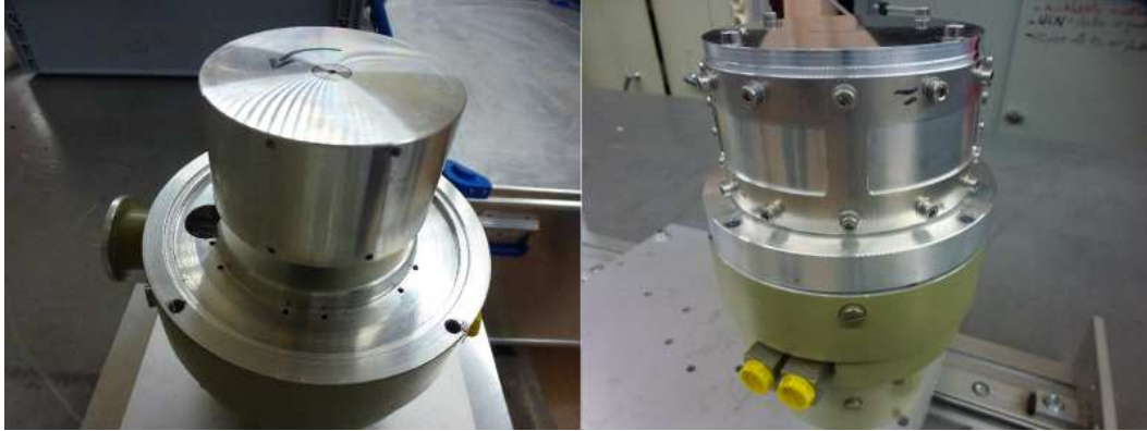
Figure 4.4.: Experimental setup with an without vacuum vessel
