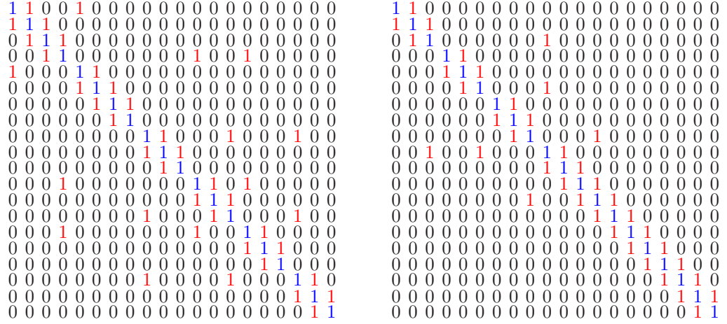
Figure 2.8: Neighborhood matrices before and after Hines ordering - (Left) The neighborhood matrix of the neuron in Fig. 2.7 with all compartments in random order. The main diagonal is indicated by blue '1'. (Right) The neighborhood matrix after the Hines ordering algorithm was employed. In the lower triangular portion non-zero elements only occur in rows of node compartments any more. Each of these far-off nonzero elements can now be eliminated in one single step, therefore the complexity of the Hines algorithm is still O(n) .
