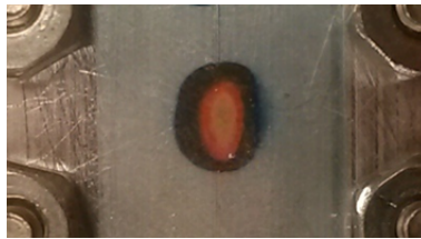
Figure 3.11: Picture of the beam spot on a radiographic film without the gold/carbon foil system. The beam spot is smaller, has no perfect circular shape and shows hot spots in the center. The orange color indicates that the film was heated over 50 °C in less than a second.
