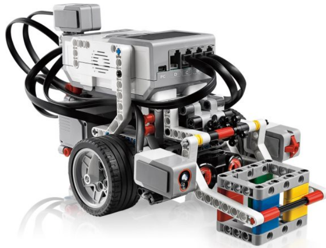
Figure 2.21: A Lego Mindstorms example which can carry objects, can move and has sensors attached.
