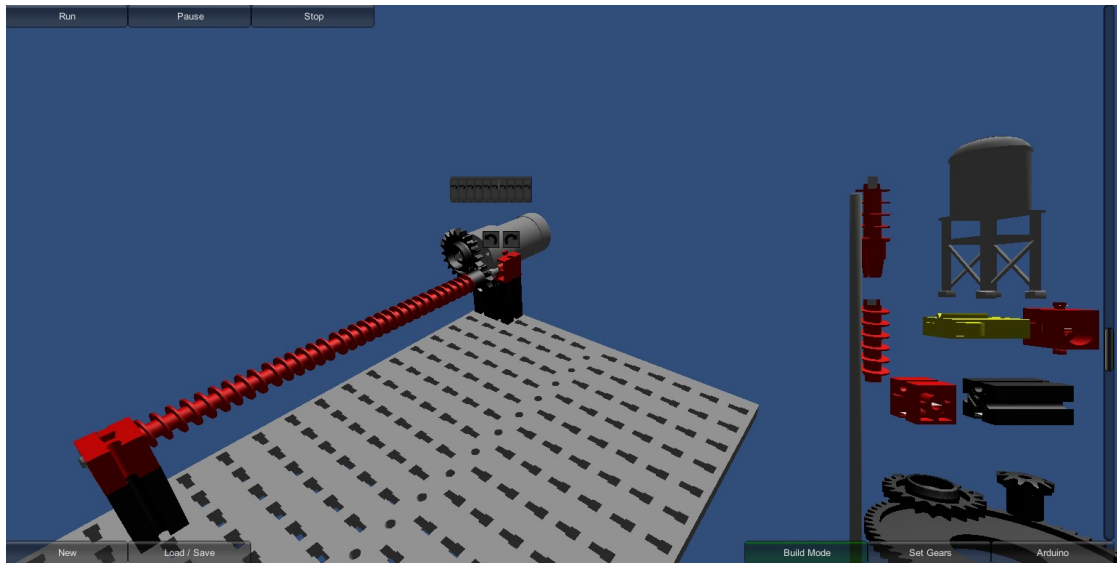
Figure 4.6: Screw threads are connected to the motor via a gear wheel.
