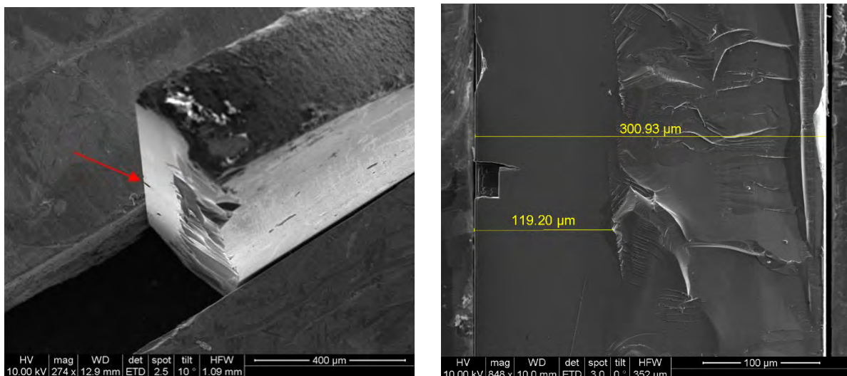
Figure 27: Left: Side view SEM picture of the Si-KE. The red arrow shows the FIB milled region, where the determination of the KE angle took place. At the same time this is the region where the experiments were conducted. Right: SEM picture showing the thickness of the cutting edge, as well as two different regions on the breaking edge face.
