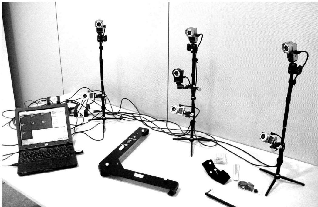
Figure 2.4: Setup of the optical marker tracking system [35] used in the audio-visual recordings. The L-shaped calibration device is visible in the lower middle of the image.
